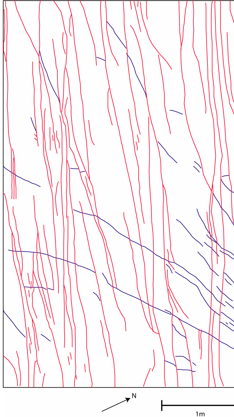
Figure 8. Wyatt pavement joint trace map. This pavement is of a sandstone unit within the Mesaverde Group located along the White River near the northern edge of the Piceance basin. The red traces outline the master joint set and the blue outline the cross set.
