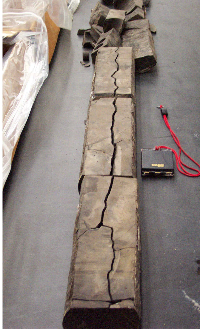
Figure 34. Picture of a core showing the joint linkage. A drilling-induced fracture is present in the center of the core with a borehole height of 4.5 m (15+ ft) with part of the fracture lying out of the field of view. Closer examination of this core indicated that this drilling-induced fracture probably exploited several smaller natural fractures, causing one large fracture.
